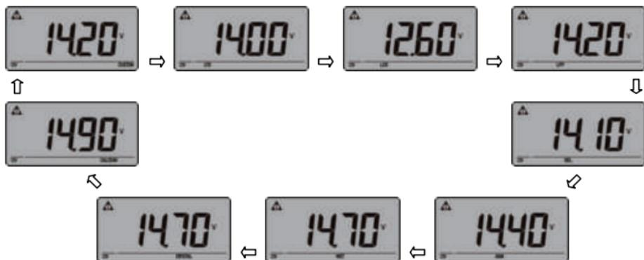
Press the **SET UP** button again, the selected battery type will be solid On and confirmed.
